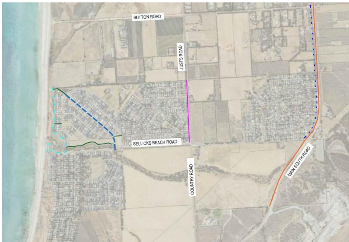
Figure 2.12: Existing and future pedestrian and cyclist links
